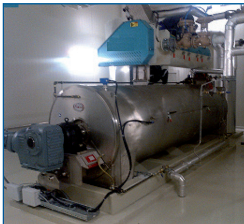
Figure 1: Steam conditioning used by Aviagen in the heat treatment of raw materials.
